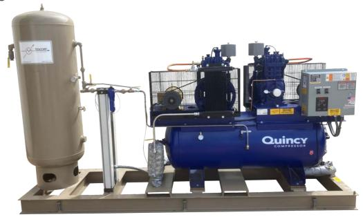
TESCORP "TIA-QR" Series systems are designed and constructed for application to meet the rugged and harsh oilfield requirements for a continuous "instrument quality" air supply with 100% redundancy for critical operation. Designed and constructed with the Quincy pressure lubricated reciprocating compressor in a duplex 100% redundant configuration, the TESCORP TIA-QR series provide continuous air supply with the capabilities to supply 200% flow rates upon demand.
