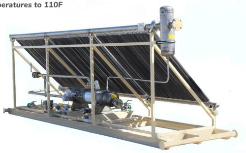
The TESCORP "BETX CONDENSER" Series systems are for application to meet EPA CFR 40, Subpart 0000 regulations and our customers' BTEX vapor recovery gas emission requirements. Designed and constructed for "wet/corrosive" gas applications utilizing all stainless steel components. TESCORP's "BETX CONDENSER" are compact, self-contained, fully-automated systems complete with gas cooling and condensing heat exchanger, pneumatic condensate controls and positive displacement pneumatic pump.
