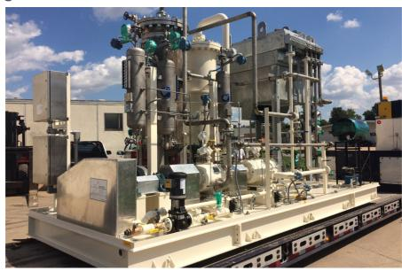
The TESCORP "CVR-2" SERIES is a completely self-contained two-stage compression system for applications for stock tank vapor recovery, flare gas recovery, or medium-pressure process gas application. Constructed with a rugged rotary vane compressor and TESCORP vapor recovery technology and components, the CVR-2 is a complete and fully-automated system for applications that require gas cooling, proportional capacity control, and sophisticated PLC driven control logic and communications.
