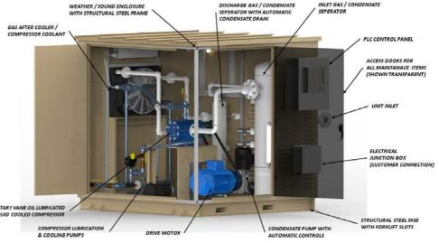
TESCORP's "CVR-MODULAR 1" VRU Series is a system for applications that meet EPA CFR 40, Subpart 0000 regulations and your stock tank vapor recovery gas emission requirements. Designed and constructed for "wet" gas applications utilizing a rugged single-stage rotary vane compressor, TESCORP's "CVR-MODULARS" are compact, self-contained, fully-automated VRU systems, complete with gas cooling, "load/no-load" capacity controls, with sophisticated PLC control logic with customer "DCS" communication.
