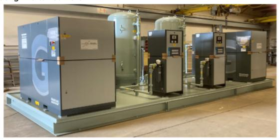
TESCORP "TIA-GA" Series systems are designed and constructed for application to meet the rugged and harsh oilfield requirements for a continuous "instrument quality" air supply with 100% redundancy for critical operation. Designed and constructed with the Atlas Copco "GA Series" Oil Flooded Rotary Screw compressor in a duplex 100% redundant configuration, the TESCORP TIA-G series provide continuous air supply with the capabilities to supply 200% flow rates upon demand.
