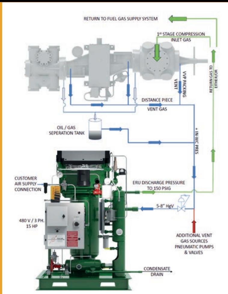
**This diagram shows how TESC Corp's ERU handles leaking emission from a reciprocating compressor. The unit uses a back-pressure regulator to maintain a positive pressure in the packing case. It then produces a slight vacuum to capture and transport all leaking emissions. Next, the ERU pressurizes the gas to meet the existing pressure inside the compressor to distribute it back into the compression process.**
